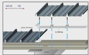
HIGHT WIND LOAD INSTALLATION DETAILING (Wind category 2 and coastal wind belt)
